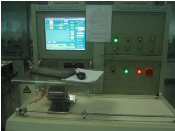
Spindle motor test
