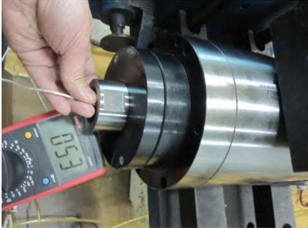
Bearing and motor interface temperature
