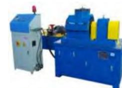
Rolling bearing fatigue life testing machine
