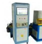
Rolling bearing material contact fatigue testing machine
