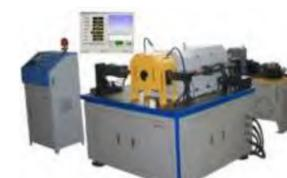
Automobile wheel bearing unit simulation test machine
