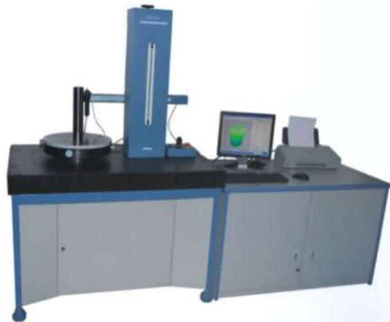
YZD-400 Ultra-precision Cylindricity & Diameter Measuring Instrument can measure roundness, cylindricity, diameter of the mechanical components by radial-method, it is widely used in many industries such as aviation, aerospace, automobile, machine, electronic, etc., it is an indispensable instrument in machining process of the precision components.
