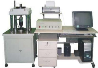
Rigidity is the capability of mechanical components to resist distortion when force is applied to it. Its value can be obtained by measuring displacement when the part is impressed by force and becomes deformed. Now in domestic, there is no specialized measuring instrument for bearing rigidity, most users just calculate bearing rigidity in theory. Some others also use simple
