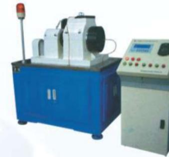
BL series rolling bearing dynamic performance measuring instrument is an mechatronics rolling bearing inspection equipment designed based on National machinery industry standards JB/T7049-93 and JB/T50093-1997. It can detect bearing vibration and temperature and assess bearing life. The instrument has reasonable design, stable performance and will not change the failure mechanism of tested bearings.
