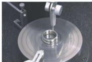
Roundness is an important indicator of production quality. The roundness value of bearing parts has a direct impact on the processing benchmark and rotary precision, noise, vibration, life expectancy, assembly quality of bearing.
