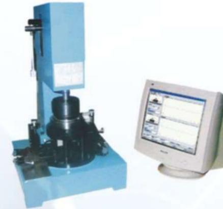
Running Accuracy is an important parameter to assess precision bearing quality. The instrument measuring principle meets ISO standard requirements, it is used to evaluate the quality of finished bearing. The instrument is also applicable to bearing check and acceptance for bearing manufacturers and military users.
