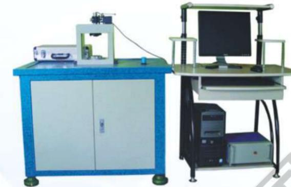
The preload of matched bearing is a key parameter. Its accuracy affects the performance of duplex bearings directly as well as the whole host. When doing the original installation, bearing will have a certain pre-deformation. So the main role of pre-load is that making the bearings skip the initial large deformation stage. It increases the support rigidity significantly. In addition, the matched bearings are used in precision shafting which needs higher accuracy.
