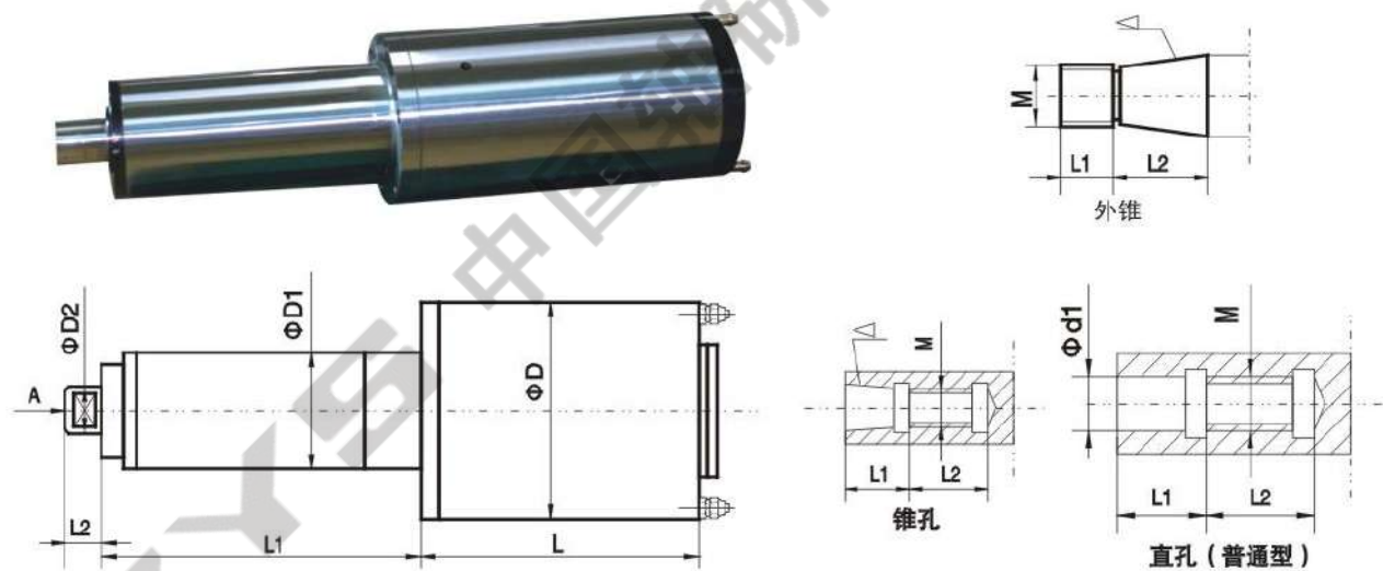
转轴与砂轮接杆联接参数 Connecting parameter between shaft and wheel bar
