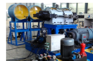
High-speed axle box bearing testing machine
