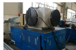
RET type bearing reliability testing machine
