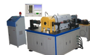
Automobile wheel bearing unit simulation test machine
