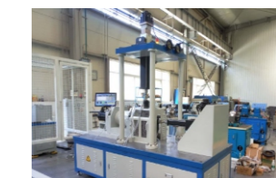
Robot RV reducer bearing testing machine
