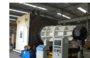
Wind power yaw pitch bearing testing machine
