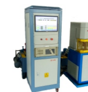
Rolling bearing material contact fatigue testing machine
