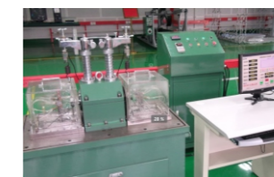
Sealed bearing waterproof testing machine
