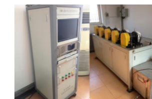
Bearing grease high temperature high speed testing machine
